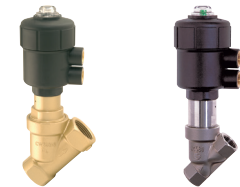
Buschjost Series 84730 & 84750 Port: 1/2", 3/4", 1", 1-1/4", 1 1/2" & 2" Pressure: 0 - 232 PSI Cv = 5.5 to 16.1 Seat Materials: NBR Materials: Brass & 316SS
